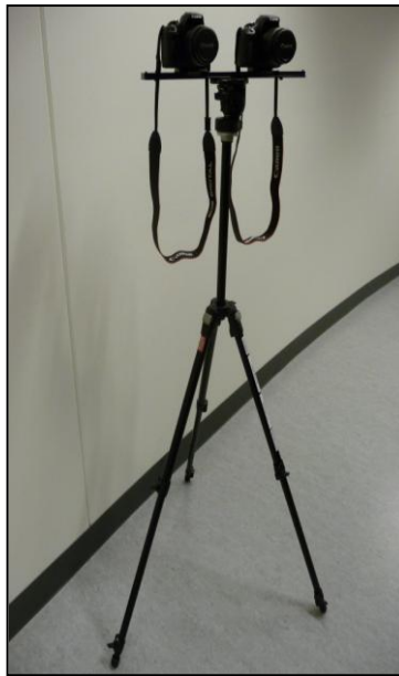
Figure 1: The camera rig, consisting of a heavy-duty tripod and Jasper Engineering precision mounting bar bearing two Canon EOS Rebel T1i 15-megapixel cameras.
