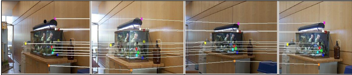
Figure 3: Automatically-detected matches across two pairs of images of the same object taken at different angles. Dots of the same color in each image represent matching points and are connected by white lines.
