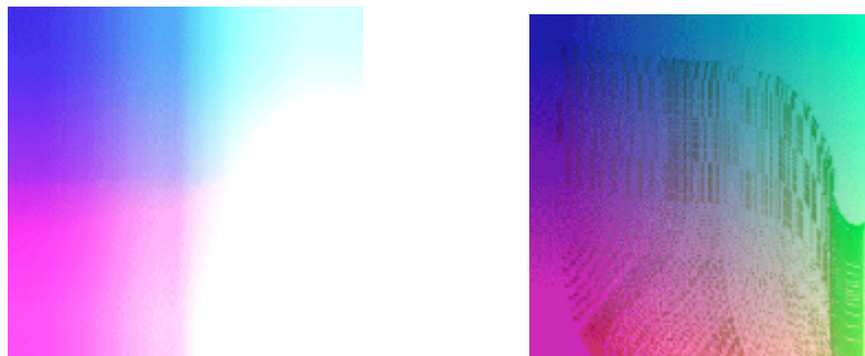
Figure 6: A cross section of the color cube created from our interpolation is shown on the left, and on the right is a cross section of the inverse color cube, where the irregular looking values are points that have data associated with them.
