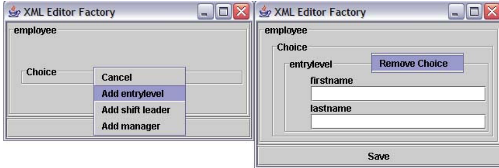
Figure 3.2.1b: Screenshots of XEF illustrating how choice indicators are handled. The user is allowed to make a choice of which element occurs with a right click menu on the left. On the right the choice has been made and a right click menu now allows them to remove the choice.
