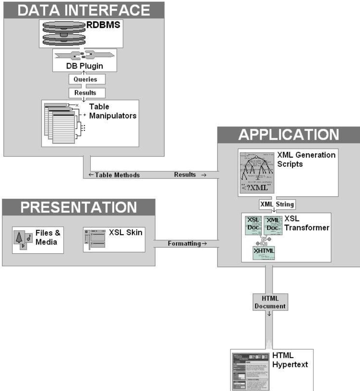
Figure 1. Layers of the modular framework
