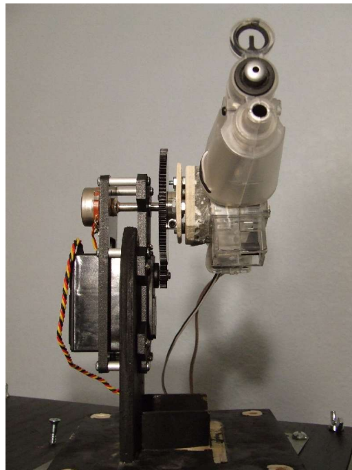
Figure 5: The AirSoft gun attached to a 5:1 reduction gearbox. The gearbox is connected to the Y actuator, which controls the elevation of the gun. The Y actuator is commanded by the BrainStem. At the bottom of the picture is the X actuator and gearbox that controls the left-right movement.
