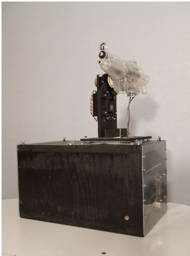
Figure 3: The entire turret assembly. The black box contains a salvaged PC power supply that powers the Airsoft gun on top, the X and Y actuators, and the BrainStem microcontroller. The BrainStem is also inside the black box.
