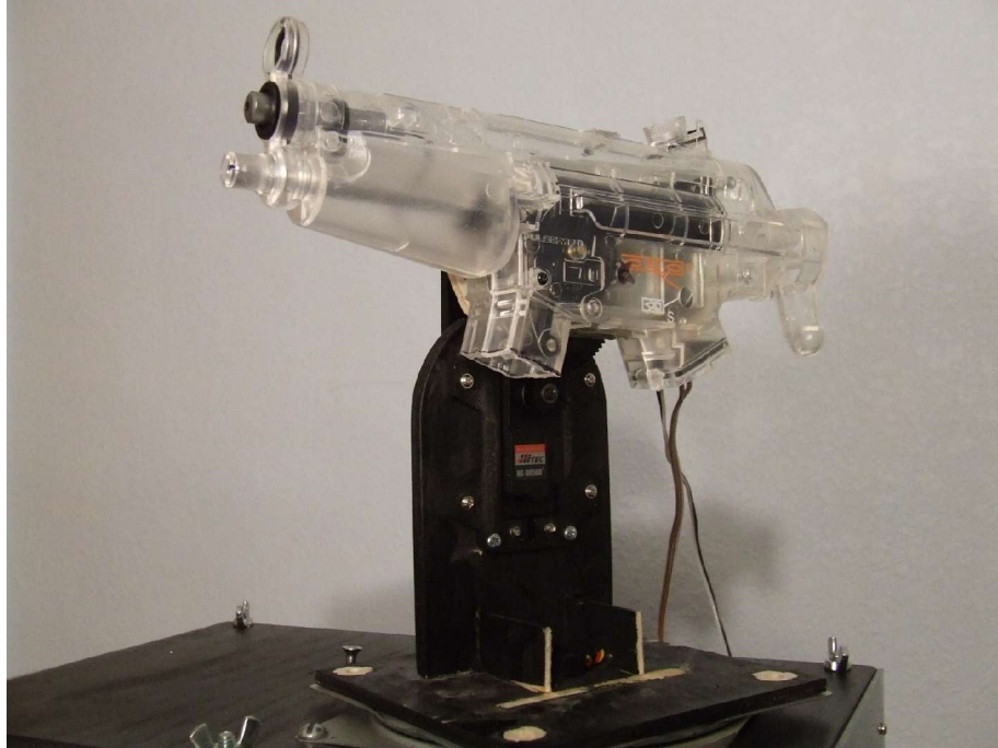
Figure 4: The AirSoft gun modified to run off the PC power supply and the trigger controlled from the BrainStem.
