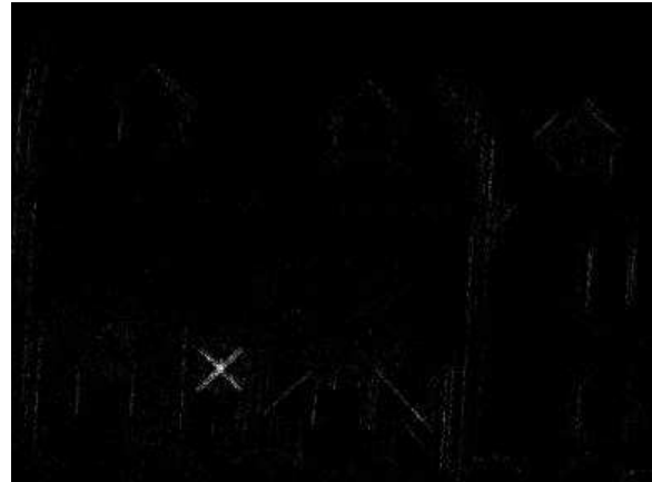
b) Accumulator array.
