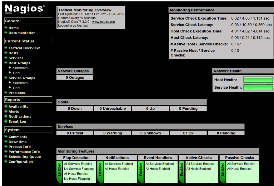
Figure 4: The Nagios Tactical Overview page. All hosts and services are performing correctly.
