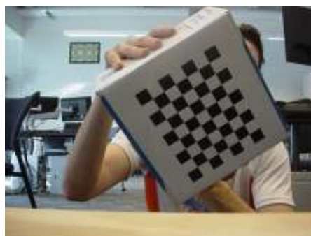
Figure 2: 8x6 internal grid calibration target.
