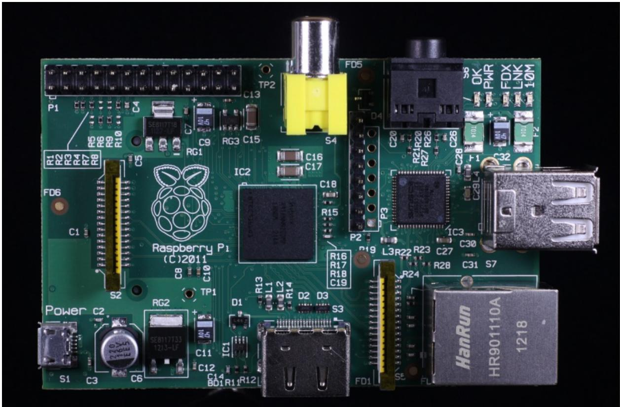
Figure 1: The Raspberry Pi main Circuit Board [2]
