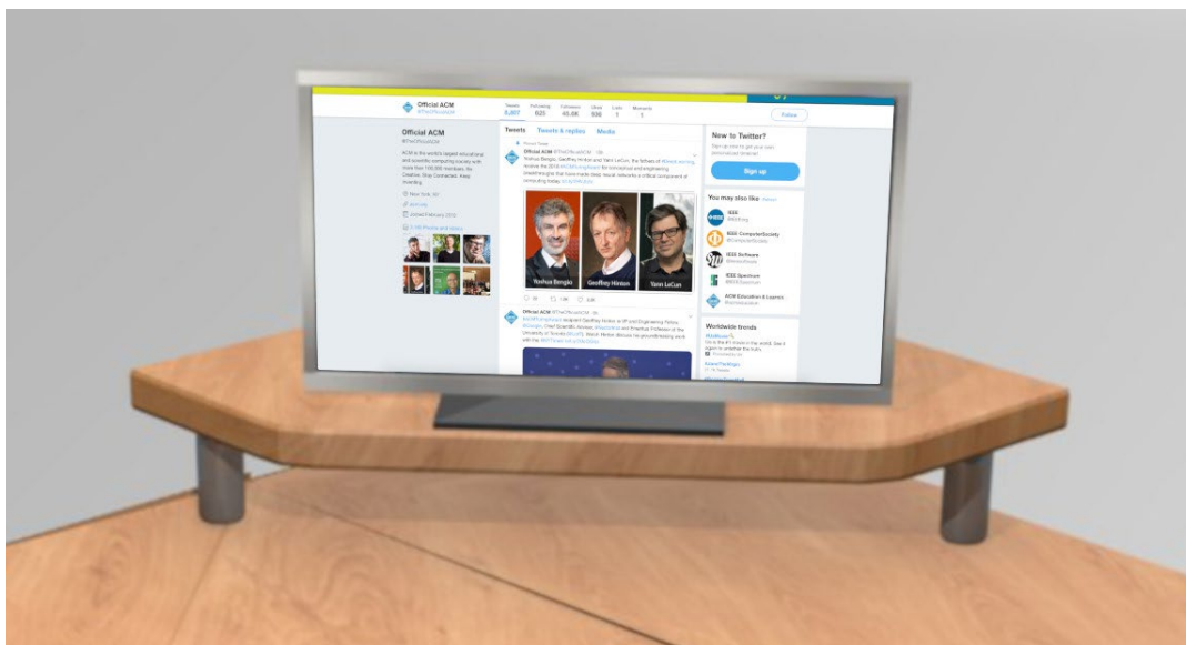
Figure 5: ACM Twitter page drawn using our web renderer embedded in 3D scene using “Desk with Computer 3D Model” [13].
