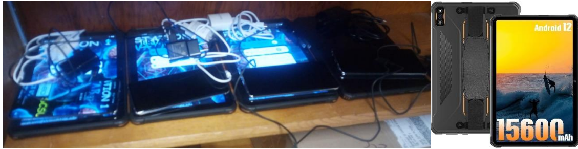
Figure 8: Tablet with MediaTek MT6762 processor, 6GB RAM, 4GB+64GB (SD up to 1TB), Cortex A73 2.0GHZ×4+A53 2.0GHZ×4,12nm process technology.
